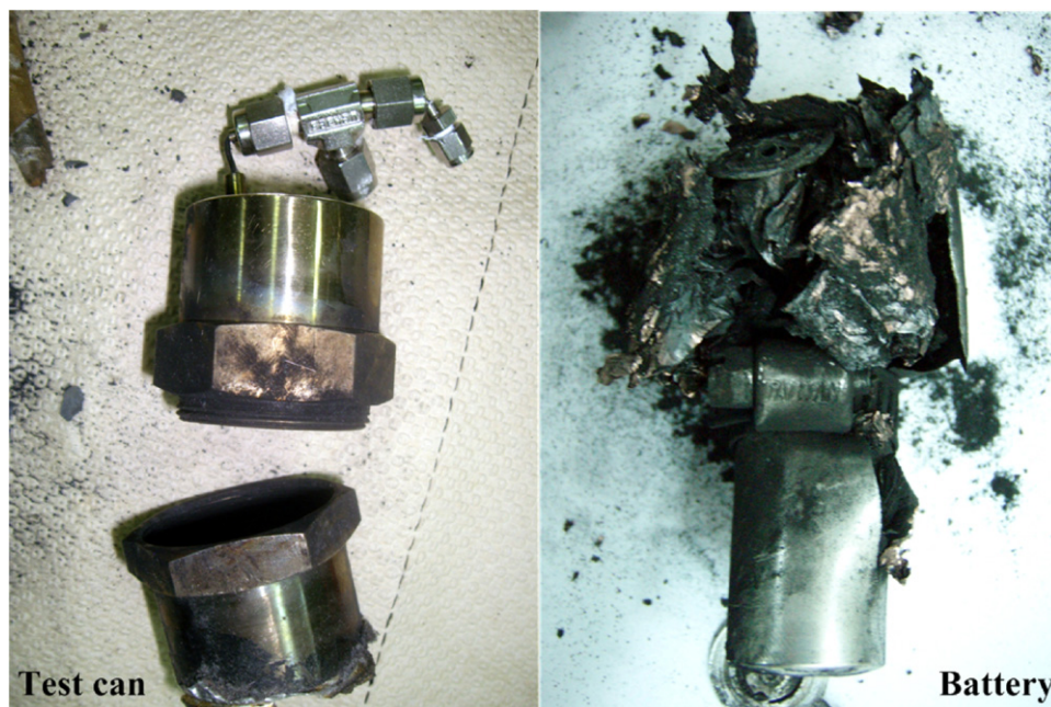
Fig. 1. The broken test can and the exploded 18650 charged Li-ion battery obtained in the VSP2 experiment without a buffer tank to relieve pressure.
